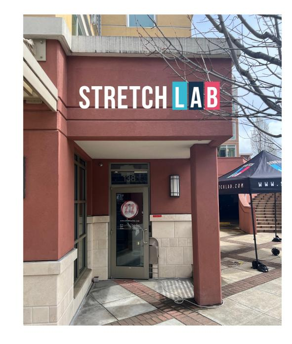
FRONT VIEW: FABRICATE AND INSTALL (1) FRONT-LIT CHANNEL LETTER SET ON RACEWAY 120V 7 amp on a dedicated
