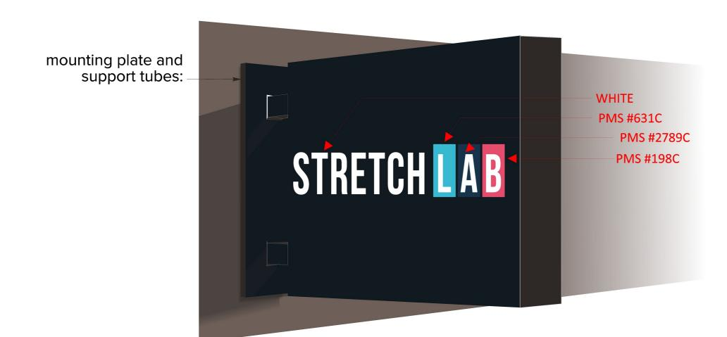
2 FRONT VIEW: FABRICATE AND INSTALL (1) NON-ILLUMINATED BLADE SIGN W/ DIGITAL GRAPHICS & LAMINATION PROPOSED SQ.FT. = 1.63 DOUBLE-FACED WEIGHT = 7
